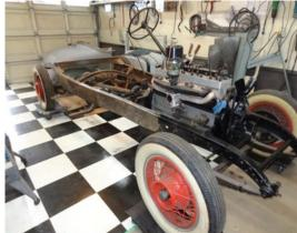
Off with the body parts (not mine I hope) as the next to be tackled is the frame. The frame wasn't too bad with the usual surface rust; the exception was that combination of 90 years old leaking oil and gravel which I classify as irremovable guck. Out comes the fire
